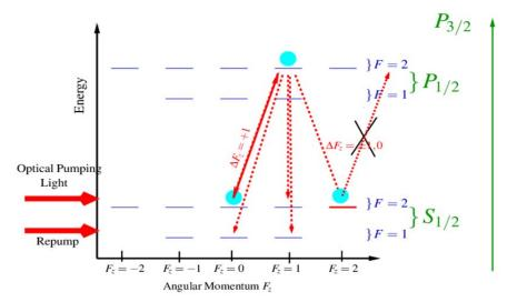
**FIG. 1.** Outline of the optical pumping process including the steps in the biased random walk. The quantum number F is the combined nuclear and atomic angular momentum. The stretched state is highlighted in red.
